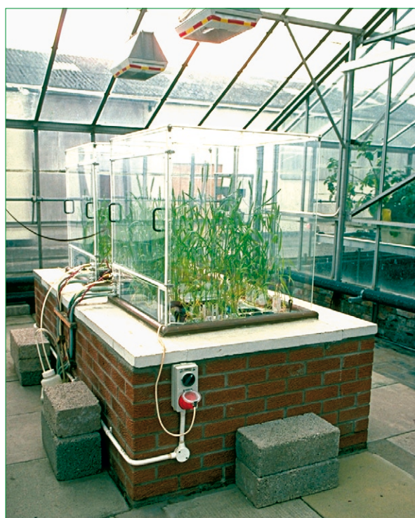
Figure 7 The climate change chambers at SCRI allow soil temperature profiles to be manipulated independently from the environment above ground, thereby creating conditions similar to those experienced by plants in the field. Environmental conditions are accurately controlled in the cabinets through a series of measurements and climatic adjustments at two minute intervals.
